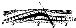
FIG. 125.—Section of a laccolith in which the feeder is along a fault-plane, to which the asymmetry of the mass is due. Lettering as in Fig. 124.
